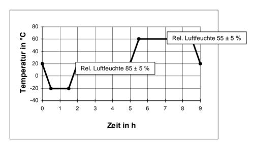
Cycle / test at alternate atmosphere
